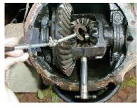
It's not necessary to remove the rear end in order to repair it. It does make it easier to clean and paint if it's removed, but this is up to you. You'll need a slide-hammer for this job too.
