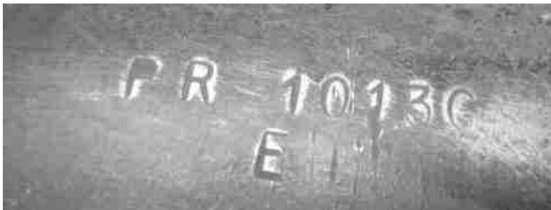
PR - 12-bolt 3.31 Positraction w/Metallic Brakes 1013 - October 13 (1966) G - Detroit Gear & Axle E - Eaton
