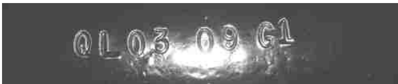
QL - 12-bolt 3.31 0309 - March 9 (1967) G - Detroit Gear & Axle 1 - 1st shift
