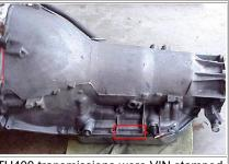
TH400 transmissions were VIN stamped either above the pan rail on the driver's side (very difficult to see with the exhaust system installed) or on the driver's side of the bellhousing (as
