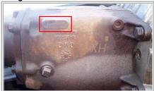
The Saginaw transmissions and the Muncie 3-speed had a pad on the passenger side of the maincase where the partial VIN was stamped. A Saginaw 4-speed transmission is shown.
