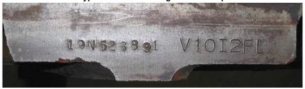
Notes: The I and 1 characters were used interchangeably in the engine code. The engine code and the partial VIN locations are reversed on big block applications.
