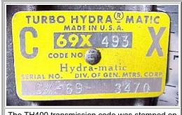
The TH400 transmission code was stamped on a metal ID plate located on the passenger side vertical surface of the transmission case. Note the CX stamp on the trans case.
