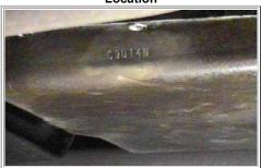
Powerglide and TH350 transmissions were stamped on the passenger side of the transmission oil pan. The front of the car is toward photo right.
