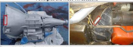
Powerglide (left) and TH350 (right) transmissions were VIN-stamped either on the forward edge of the bellhousing on the driver side or on a pad on the passenger side.
