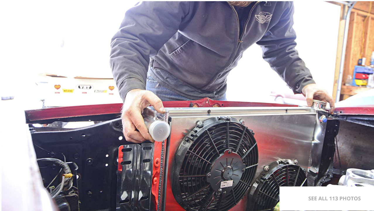
We took the opportunity to clean and paint the radiator support before sliding the new Frostbite radiator and shroud assembly into place. It is designed to use the original bolt holes in the radiator support.
