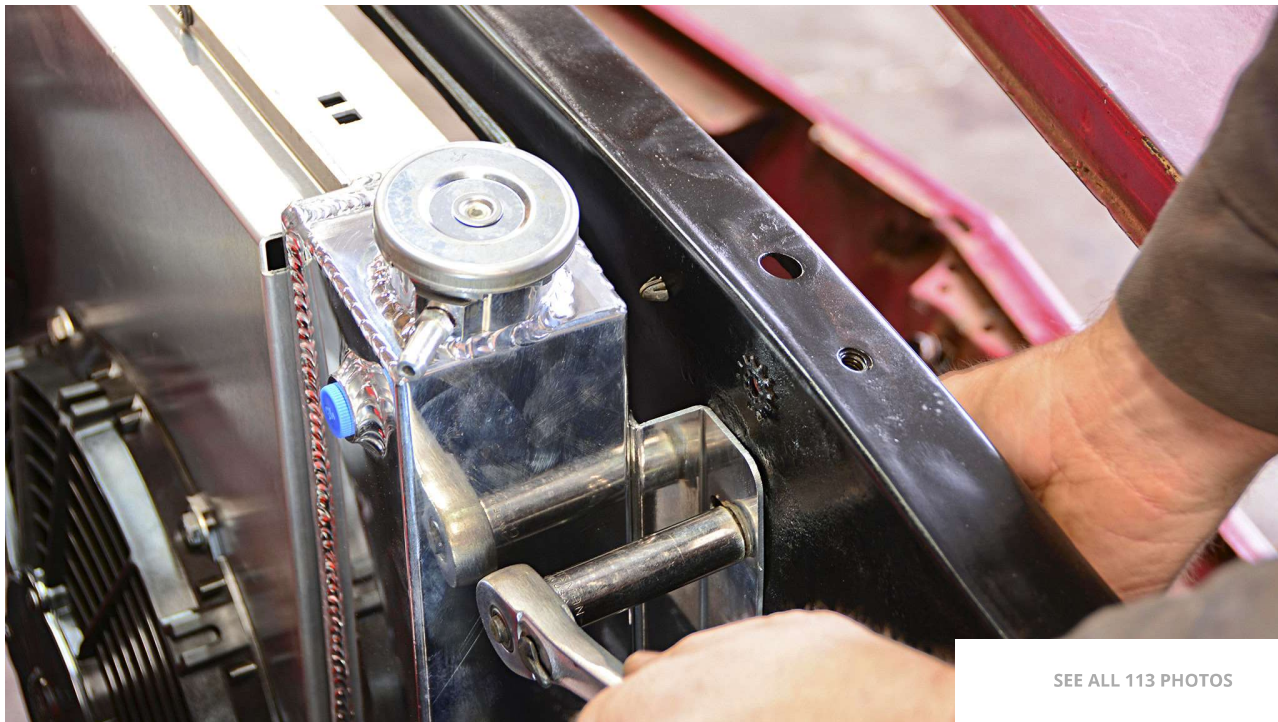
Installing the radiator is as simple as tightening four bolts. The position of the new Frostbite radiator is the same as original so all of our original-style lines and hoses can be installed easily.
